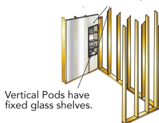
Vertical Storage Pod Install with a Header Top & Bottom
