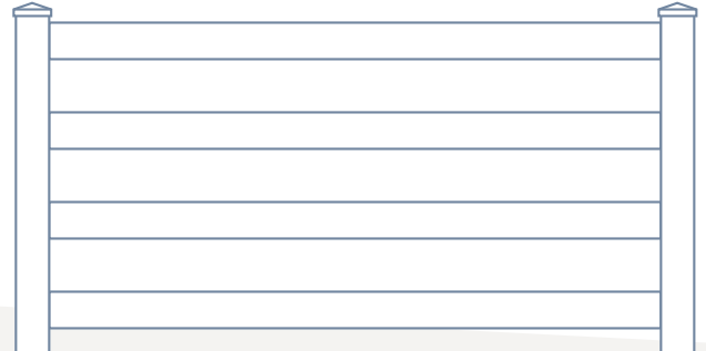
Approximately 8-1/4" space between rails
